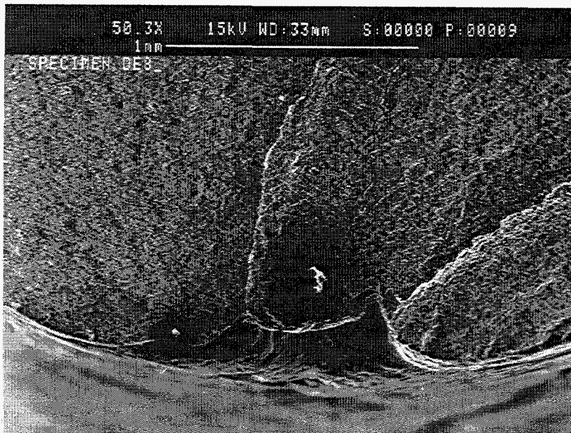
Figure 5.22. (A) Typical fracture Face of As-cast EPC Ductile Iron Specimen. 10X (B) SEM Micrograph Showing Bead Intersection Notch on As-cast EPC Ductile Iron Specimen. 50.3X
