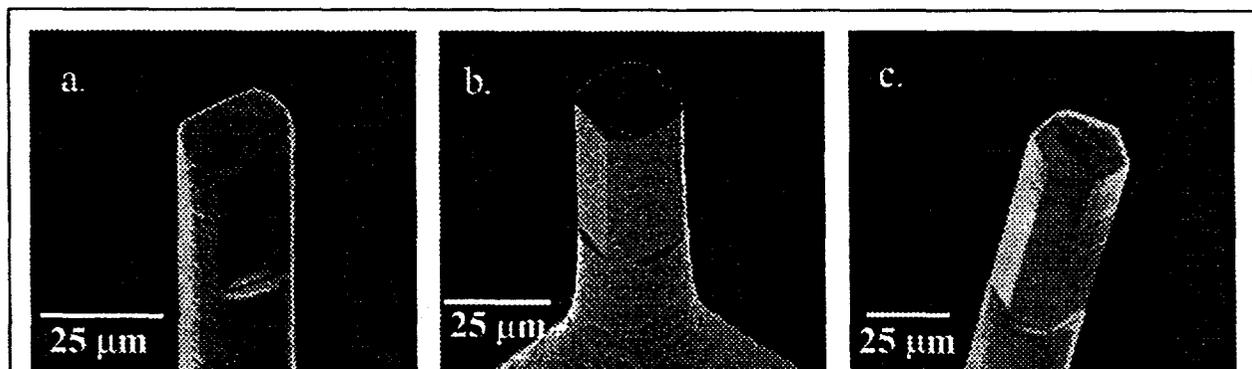
Figure 1. SEM micrographs of micro-end mills made with focused ion beam sputtering. Tools have 2, 4 and 5 cutting edges.
