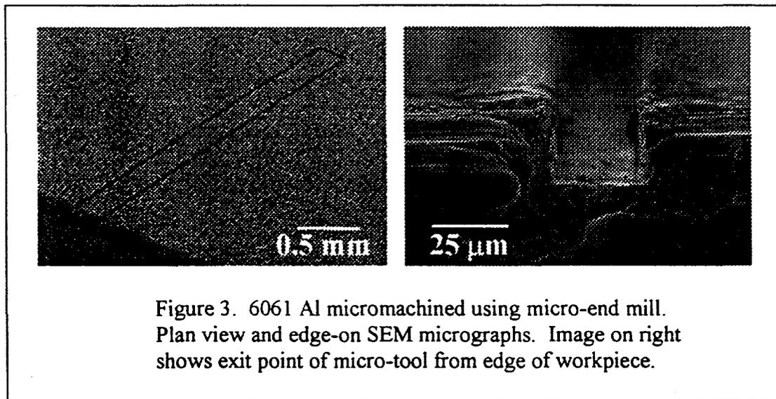
microscope during micromachining of 6061 Al (without lubricant) demonstrates that these tools cut, not burnish. We observe chip removal for feed rates of  $2\text{mm}/\text{minute}$  and  $18,000$  rpm using 2-facet micro-tools.
