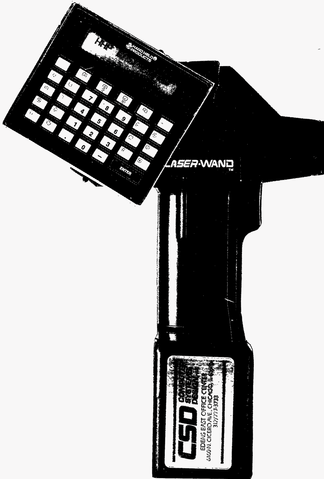
Fig. 10. Combination Standoff Bar-Code Reader and Computer (Laser Wand from Hand-Held Products)
