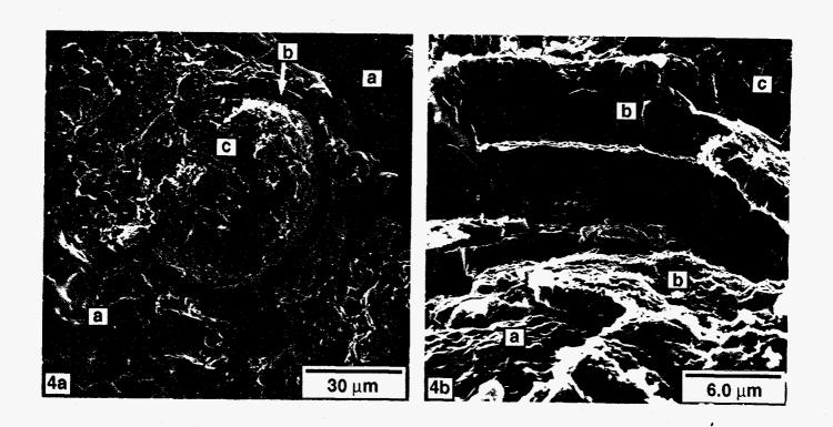
Fig. 4. (a) Secondary electron images of the substrate side of the YSZ failure surface after thermal cycling, showing: (a) YSZ remaining adhered to the majority of the bond coat surface, (b) cross-sectional fracture surface of the interfacial scale, and (c) protruding NiCrAlY surface particle covered by a cracked subscale.
