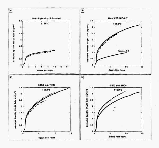
Fig. 1. Parabolic plots of the isothermal oxidation weight gains at  $1150\,^{\circ}$ C in dry air for (a) bare Rene'N5 (with as-machined surfaces), (b) bare VPS NiCrAIY, (c) 250  $\mu$ m TBCs, and (d) 500  $\mu$ m TBCs. The surface area of a flat substrate was used to calculate all specific weight gains.
