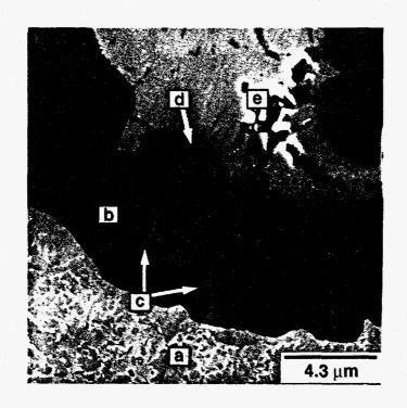
Fig. 3. Secondary electron micrograph of the bond coat/top coat interface of a Type-C TBC specimen after 200 hours at 1150°C. The features labeled are: (a) bond coating, (b) Al<sub>2</sub>O<sub>3</sub> scale, (c) alumina-yttria particles, (d) Ni(Cr,Al)<sub>2</sub>O<sub>4</sub> spinels, and (e) YSZ top coating.
