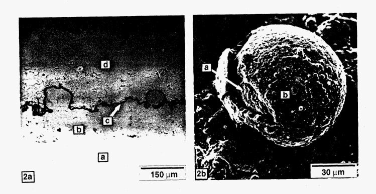
Fig. 2. Secondary electron images of: (a) Type C TBC cross-section after 200 hours oxidation showing the (a) substrate, (b) bond coat, (c) interfacial scale, (d) YSZ. Note the bond coat interface roughness and the spherical surface particles interlocked with the YSZ. (b) Spherical particle on a bare NiCrAlY surface after 100 hours isothermal oxidation showing (a) bare NiCrAlY, and (b) scale which has cracked and partially spalled.
