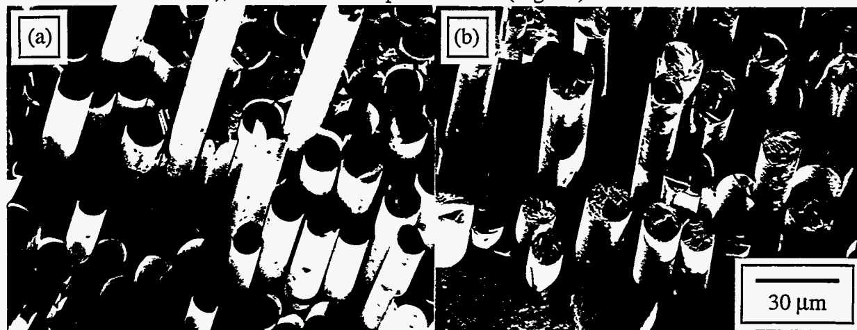
Figure 6. The fracture surface of a SiC/Nicalon tested at 600°C for 20 h; a) graphite interlayer removal in the tensile region and b) interlayer retention in the compressive region.
