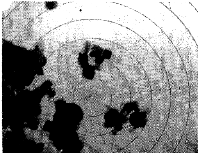
Figure 12. TEM @ 78,000x, LaNiO 3 , HCP Process, 700°C, 6 hrs, with Na 2 CO 3 as Sintering Interferant; 14 m 2 /g (N463-17-28A)
