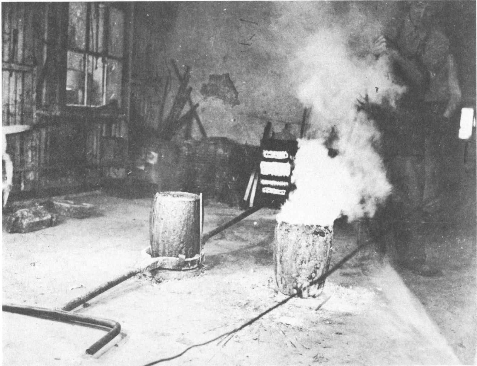
Figure 3. - Nonferrous crucibles, one with cover, other without.
