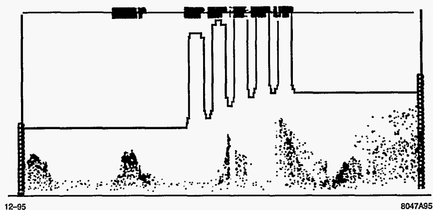
Figure 8-33. Computer simulation of bunched beam passing through the X5011 disk-loaded output circuit. The vertical scale is magnified by 3 to emphasize the growth of bunch amplitude in the output circuit.
