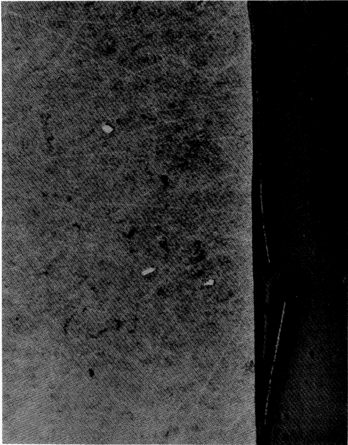
Figure 3.16: Photomicrograph, 250X, of the As-Polished Conditioned Specimen SFEC5,4378-S2-B in the Longitudinal Plane Illustrating Spalling Off of the Oxide Layer. PTL Log Q-1508, Photo # 326.
