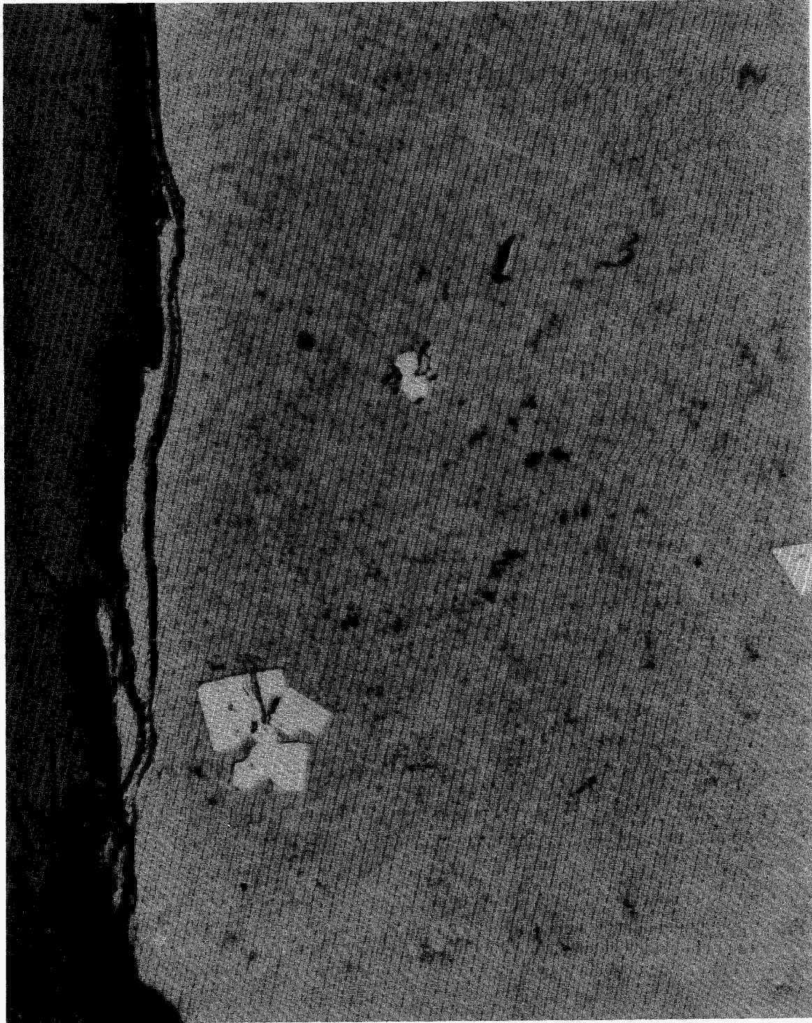
Figure B.61: Photomicrograph, 250X, of As-Polished Conditioned Specimen SFEC5,4378-S2-B in the Longitudinal Plane. The photo illustrates formation of loose oxide layer on the cut uranium surface. PTL Log Q-1507, Photo # 325.
