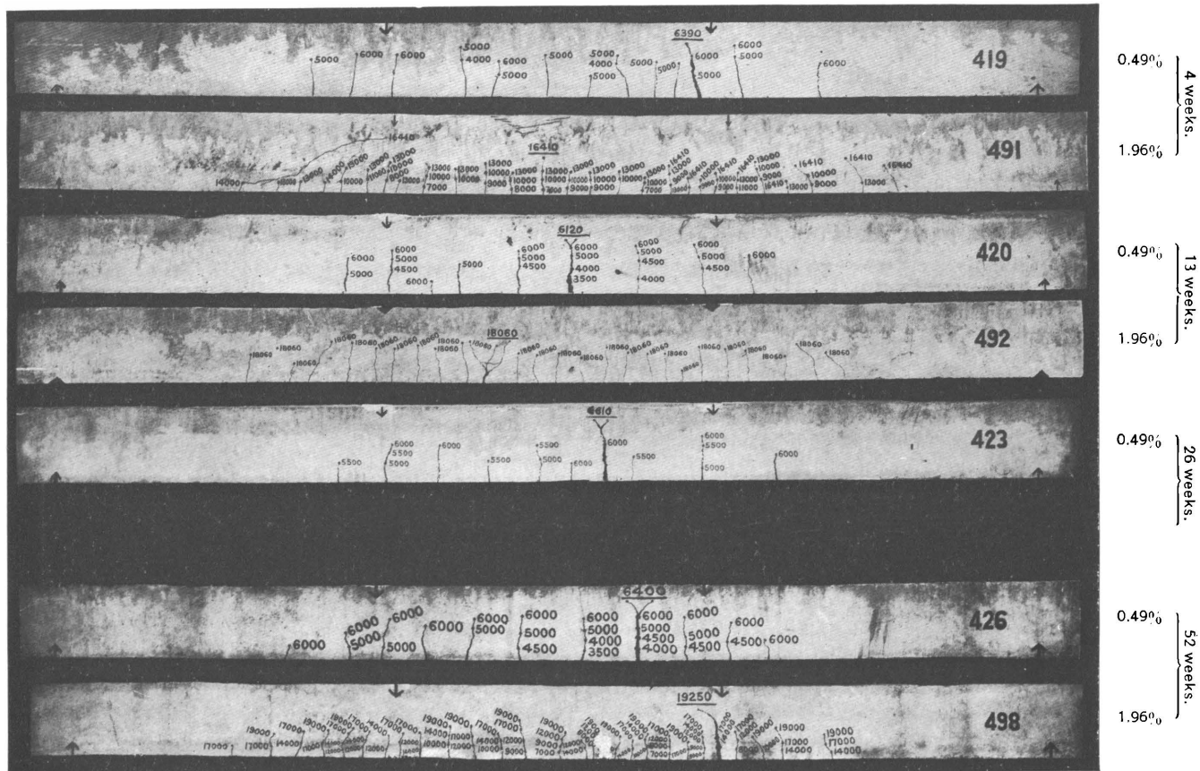
Fig. 29.—Cinder Concrete, Showing Beams with 0.49 and 1.96 Percentages Reinforcement
