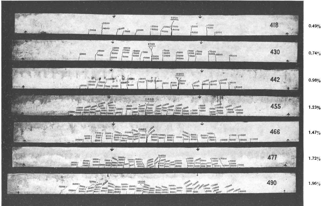
Fig. 25.—Cinder Concrete, Age 4 Weeks, Showing Variation in Position of Cracks with Variation in Percentage of Reinforcement
