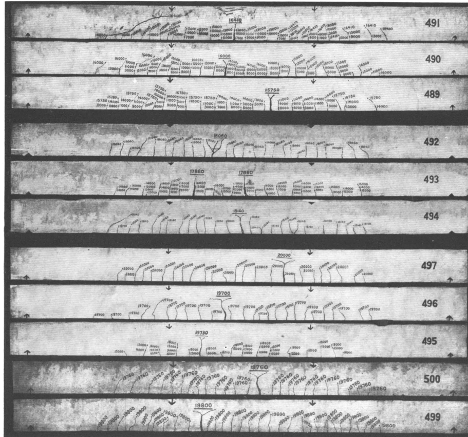
Fig. 30.—Showing Similarity of Cracking in Similar Beams
