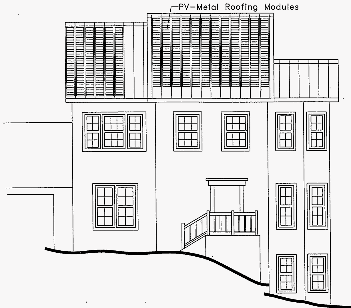
Figure 6 Townhouse Diagram with PV-Metal Panels
