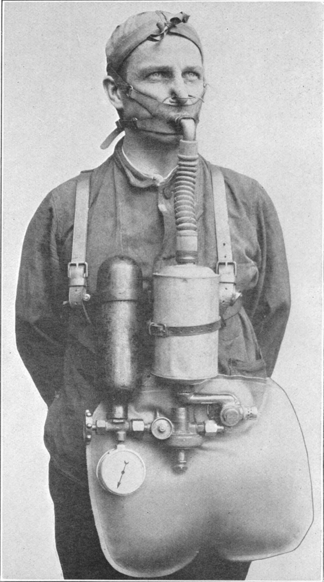
SALVUS LIGHT APPARATUS; SUPPLIES OXYGEN FOR HALF AN HOUR AND WEIGHS ABOUT 15 POUNDS.
