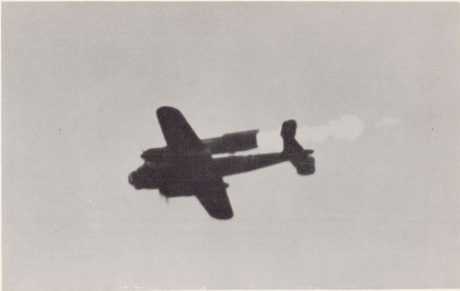
Figure 28.- 20,000-hp jet tube on the Do 217E7 with v = 130 m/sec in operation.
