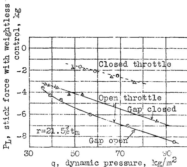
Figure 5.- Stick forces by open and closed gap.
