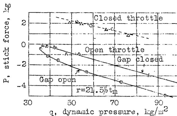
Figure 6.- Stick forces when assuming weightless control, showing those set up exclusively by the air loads on the tail.
