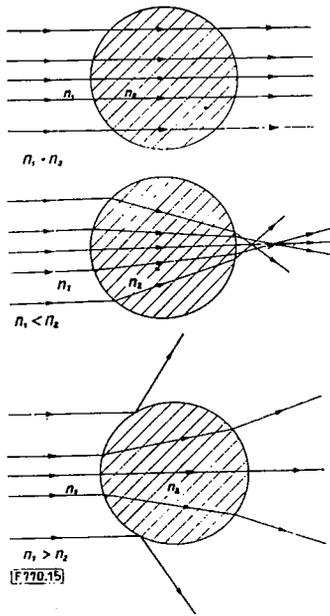
Figure 15.-Refraction of light at the boundary between two media having different refractive indexes  $n_1$  and  $n_2$ .
