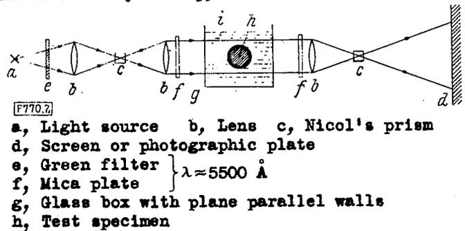
Figure 2.- Apparatus for the photo-elastic investigation of three dimensional stress and strain conditions.
