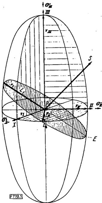
Figure 1.-Fresnel's ellipsoid. It characterizes the propagation of light in any small deformed particle of a transparent substance.
