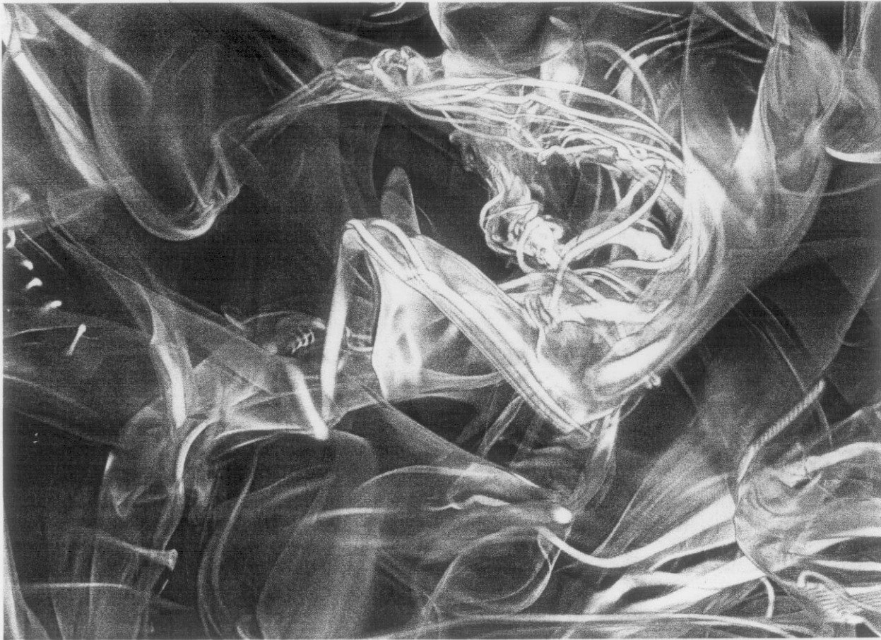
Figure 5. The distribution of the magnitude of vorticity is visualized in this volume rendering of a region of the billion-cell simulation of homogeneous, Mach \frac{1}{2} turbulence. Near the center of the figure, a group of thin vortex tubes are spiraling around each other as a whole section of a vortex sheet rolls up. At the left, a series of roughly parallel vortex tubes is intensifying out of another vortex sheet. This visualization captures the developing turbulent flow in the midst of its transition from a state dominated by vortex sheets to one in which such sheets can no longer be identified within the dense tangle of spaghetti-like vortex tubes.
