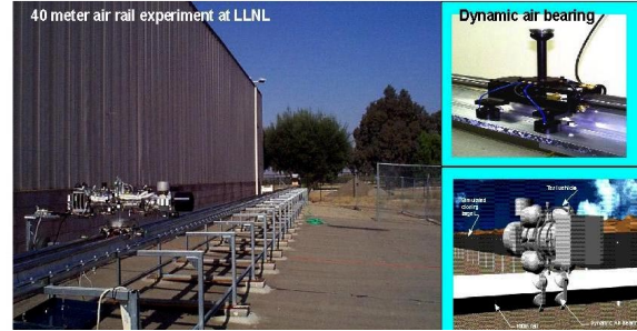
Figure 10 Warm gas DACS stabilized and propelled the vehicle during testing.
