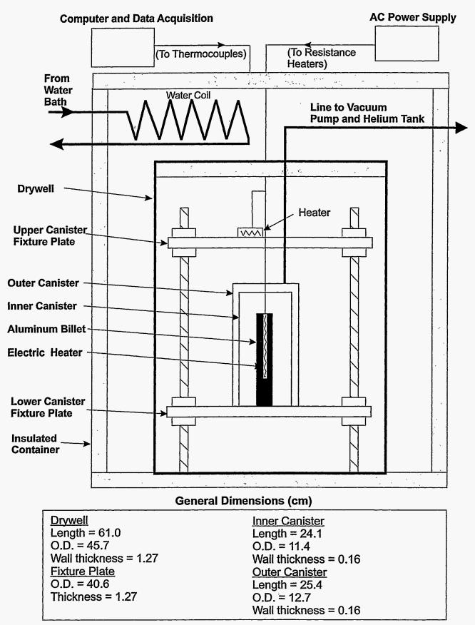
Figure 2. Schematic diagram of the NMSF single nested canister experimental apparatus.
