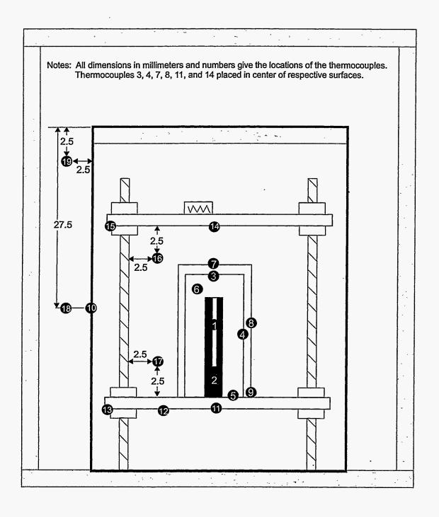
Figure 3. Schematic diagram of the thermocouple locations on the single nested canister experimental apparatus.
