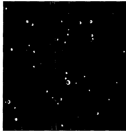
Fig. 7b. SEM photomicrograph showing particulates formed with 90% density target.
