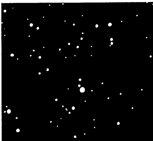
Fig. 6a. SEM photomicrograph showing particulates formed with pulse width of 27ns.
