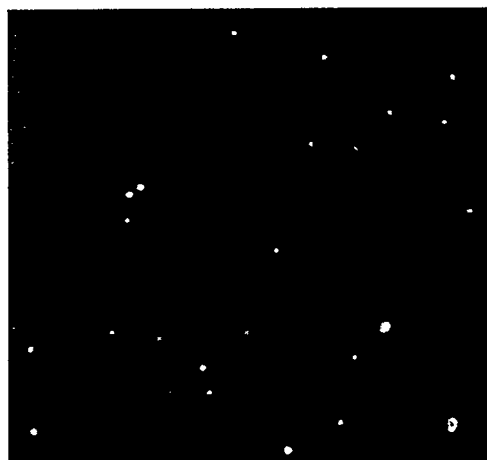
Fig. 6b. SEM photomicrograph showing particulates formed with pulse width of 16ns.
