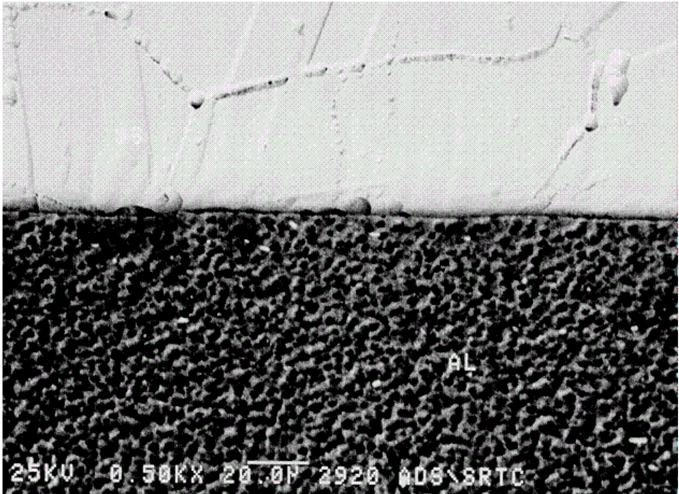
Figure 13. SEM of mounted and etched 6061 T6 Al to 304L stainless steel inertia welded specimen.
