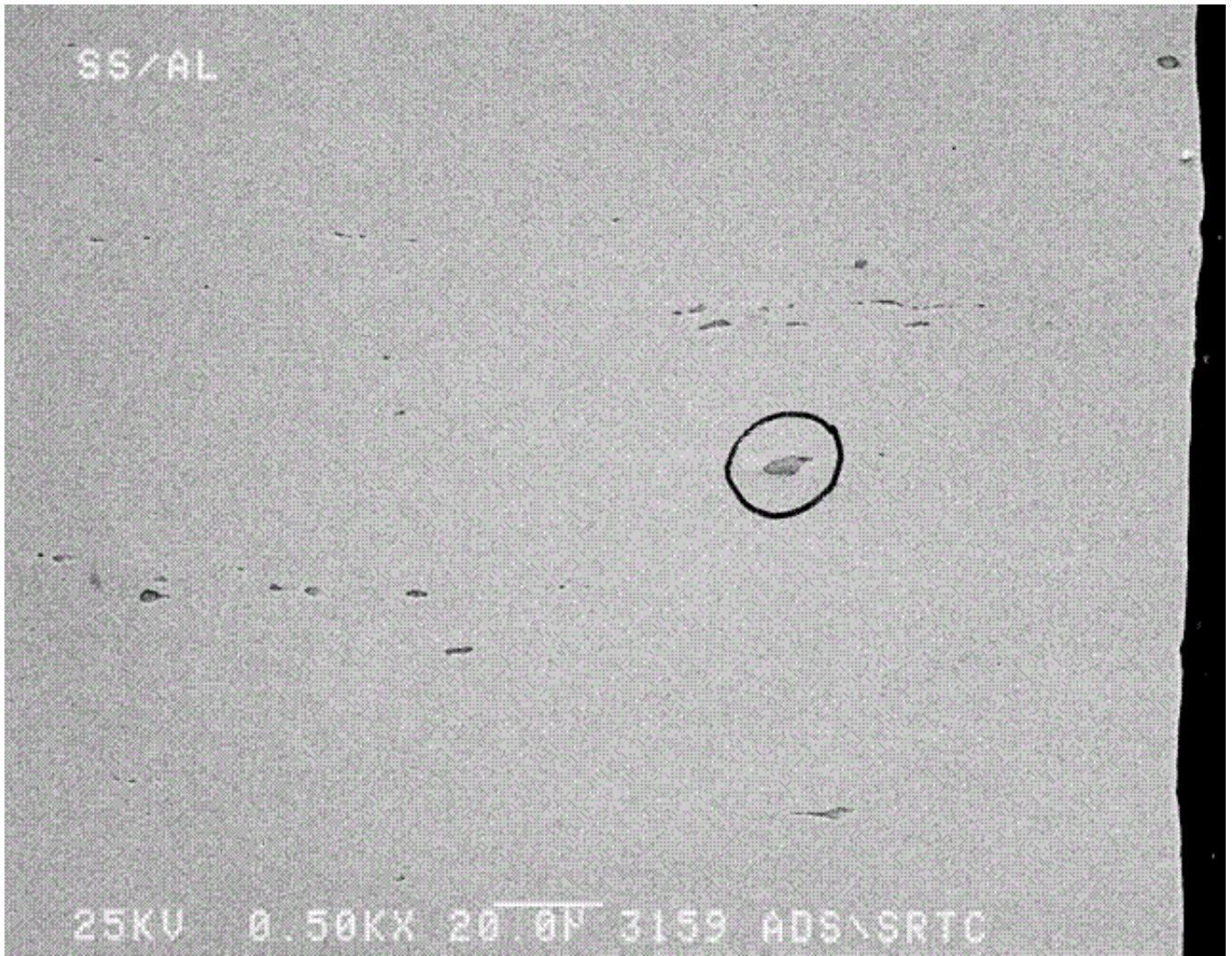
Figure 14. SEM photograph of stainless steel portion of inertia welded specimen in the unetched condition. Page 28 bottom
