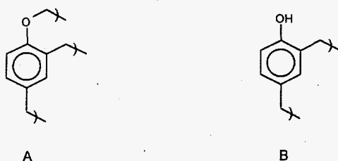
Figure 4-19. The Two Structural Components of Duolite CS-100 Resin: A - 54.8%; B - 45.2%
