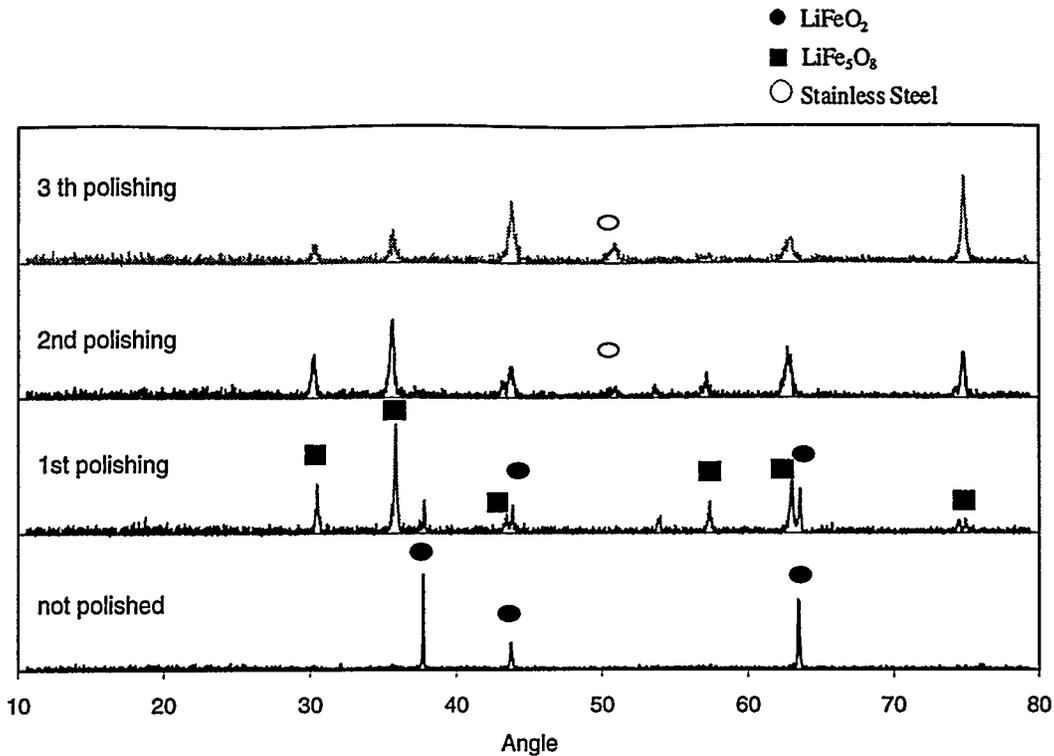
Figure 6 shows a typical XRD pattern through the oxide scales of 316L using (Li,K) electrolyte with an outer  $\text{LiFeO}_2$  layer. For stainless steels, which contain between 16-18 %Cr, an outer layer is built from  $\text{Fe}_2\text{O}_3$ , which is formed in the first few hours (1). Marker experiments have shown that the outer layer mainly grows by outward iron diffusion (1):
