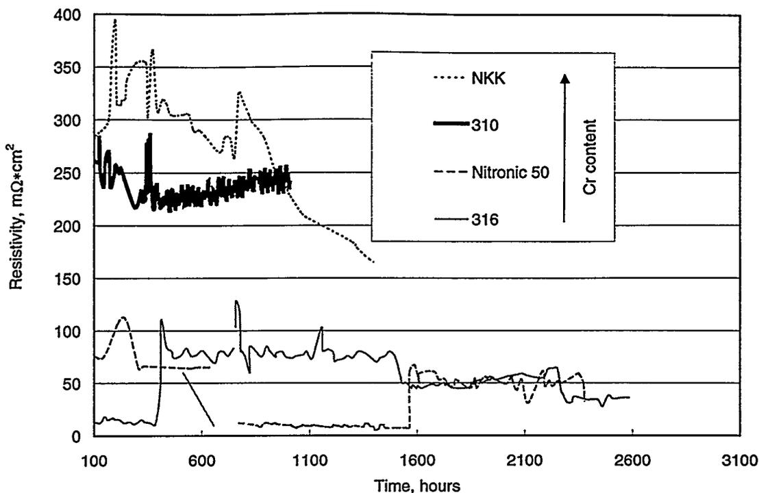
A key factor for the electrical resistivity seems to be the phase composition of the inner or intermediate oxide scales which are formed under MCFC conditions. The composition of the inner corrosion layer varies with chromium content of the base metal. Both 310S and NKK have an inner  $\text{LiCrO}_2$  layer, which may lead to high resistivities. Additionally, we found porosity between the oxide scale and the base metal of NKK, which explains its rather high interfacial resistivity.
