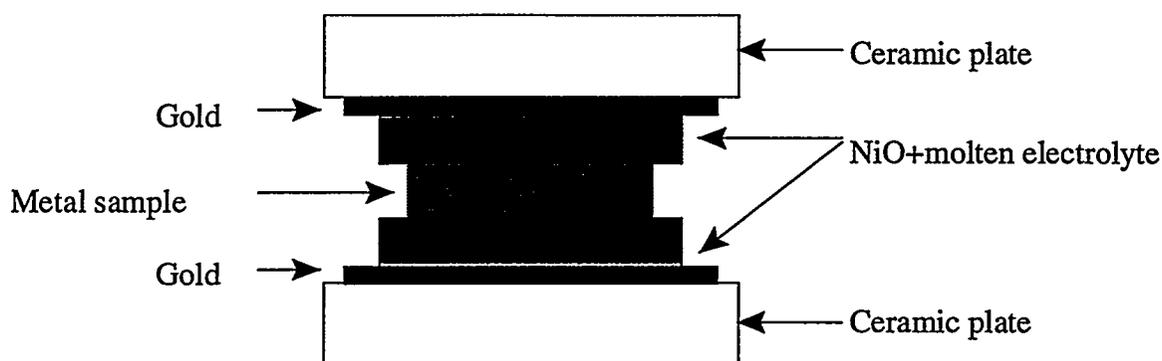
Corrosion tests were carried out in a cathodic environment (30 %CO<sub>2</sub>/air) at 650°C for different exposure times. Afterwards, the samples were mounted, ground, polished, and subjected to microstructural measurements in order to characterize the corrosion behavior. Scanning electron microscopy (SEM) and energy dispersive X-ray spectrometry (EDX) were carried out on metallographic cross sections to determine the thickness and composition of the oxide scale.
