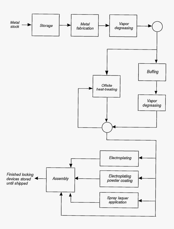
Figure 1. Abbreviated process flow diagram for locking device fabrication.
