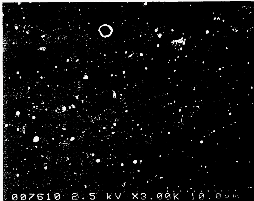
Figure 3. Secondary scanning electron image of a transverse cross section of ODM-331 showing the small grain size and the presence of cavities and oxide particles.
