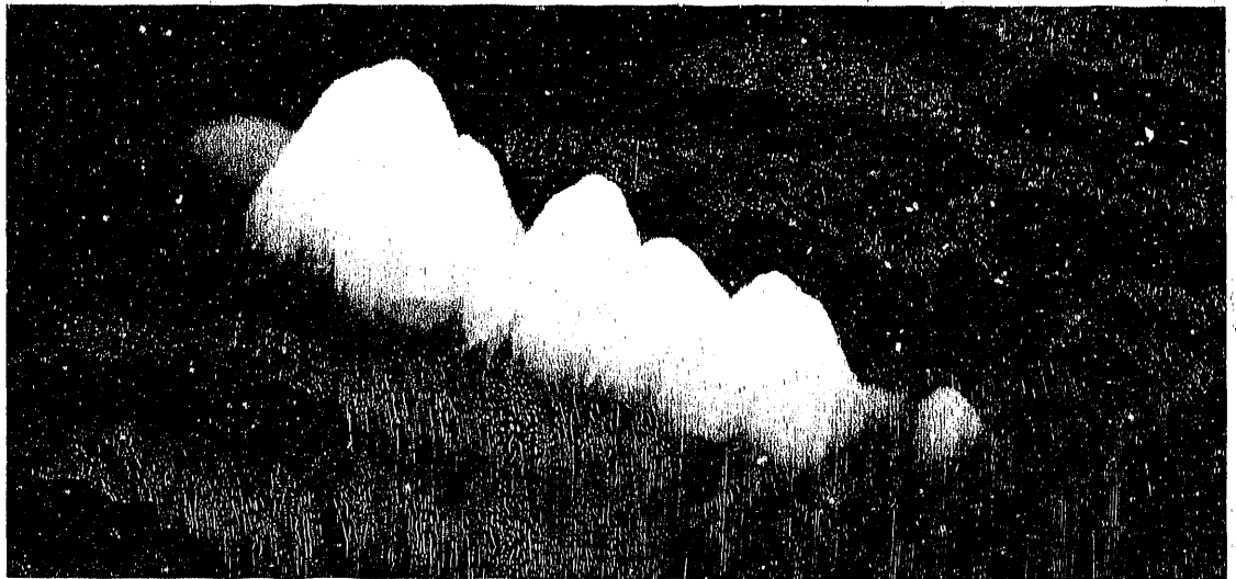
Topographic image of DNA obtained by scanning tunneling microscopy
