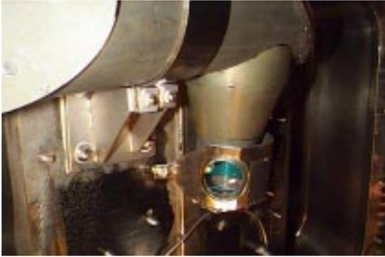
Figure 1. View of MSE from inside C-Mod showing input lens, vertical housing for second lens set, split ring support, and thin wall housing containing last two mirrors.
