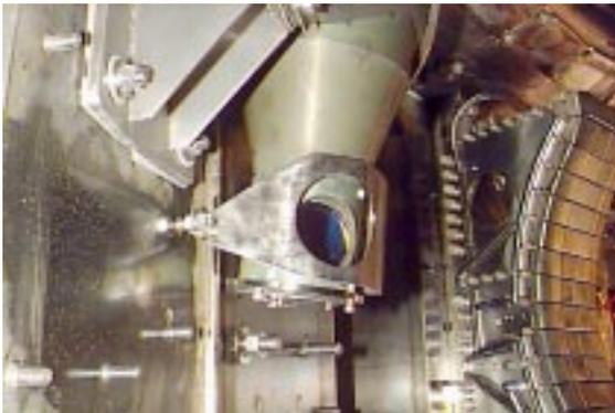
Figure 2. Close-up view from inside C-Mod of MSE showing input lens, heat shield and lower portion of split ring support bracket.
