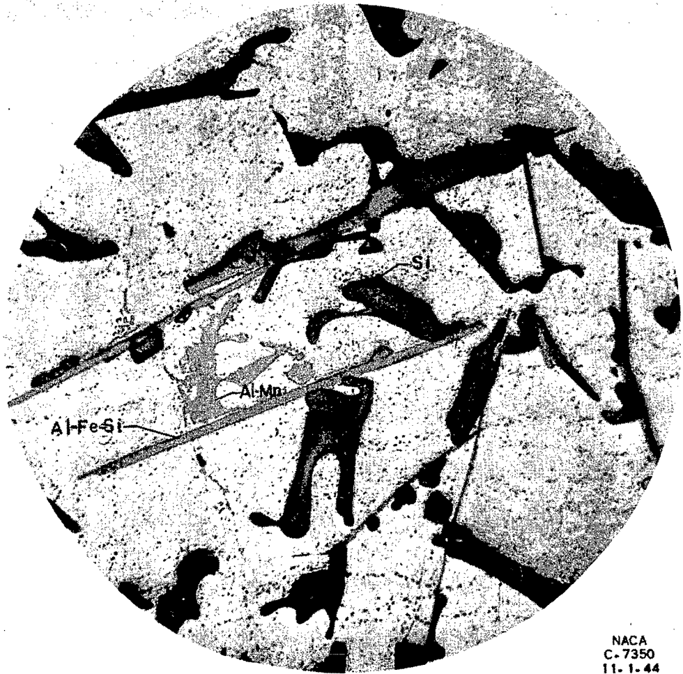
(a) From top of impeller 2-23. Etched in hydrofluoric acid.
