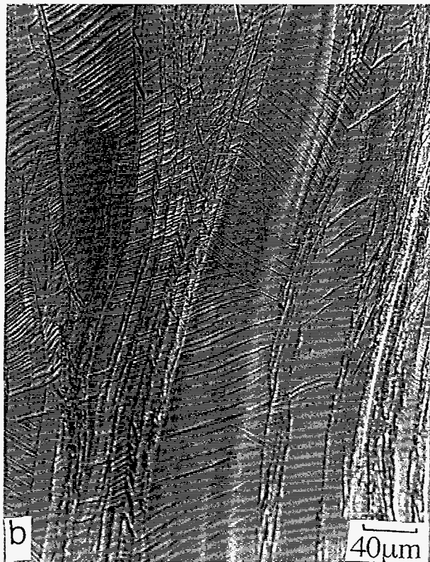
Fig. 7. Comparison etches on a Ti-60 Ta specimen using (a) new chemical polish and etch procedure. Light micrographs, ASTM etchant #192, (b) ASTM etchant # 178, and (c) the not ext interference contrast line.
