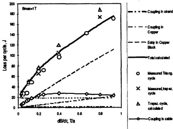
Fig.2 Losses in parallel field, 1 T cycle
