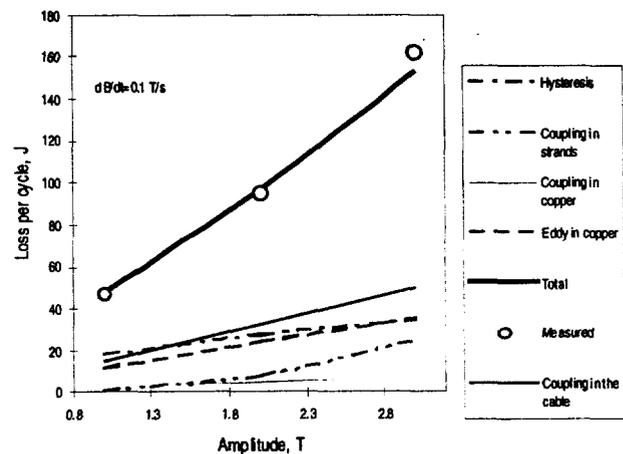
Fig.3 Losses in parallel field,  $dB/dt=0.1$  s
