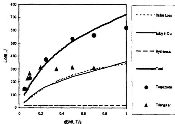
Fig.6 Losses in ITER transverse field, 1 T trapezoidal cycle, long flat top (triangular cycle measured losses are shown for comparison)
