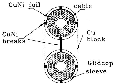
Fig. 1. Cross section of the US PP joint
