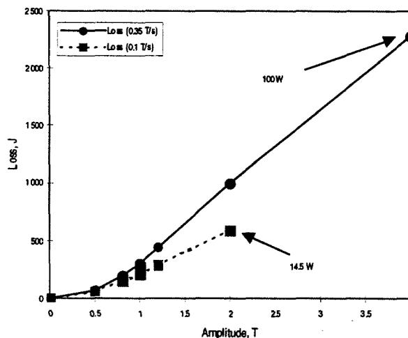
Fig.7 Losses in transverse field, triangular cycle
