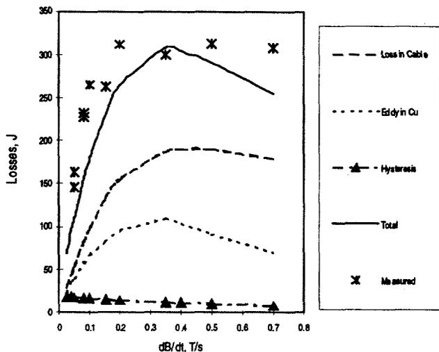
Fig. 5 Loss in ITER transverse field, the 1 T triangular cycle, calculated versus measured
