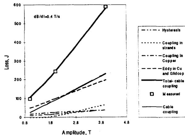
Fig.4 Losses in parallel field,  $dB/dt=0.4$  T/s
