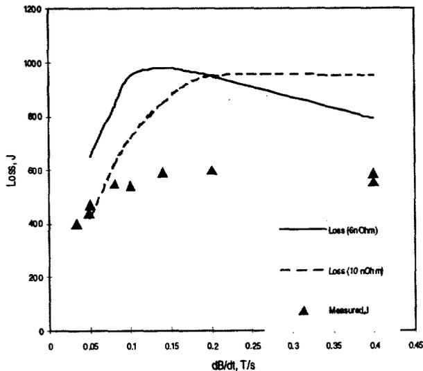
Fig. 8 Non-ITER field losses, calculated versus measured, 1 T triangular cycle
