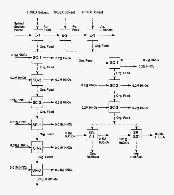
Figure 4. TRUEX flowsheet tested in 5.5 cm centrifugal contactors.
