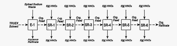
Figure 3. Procedure for evaluating mercury in a simulated TRUEX process flowsheet.
