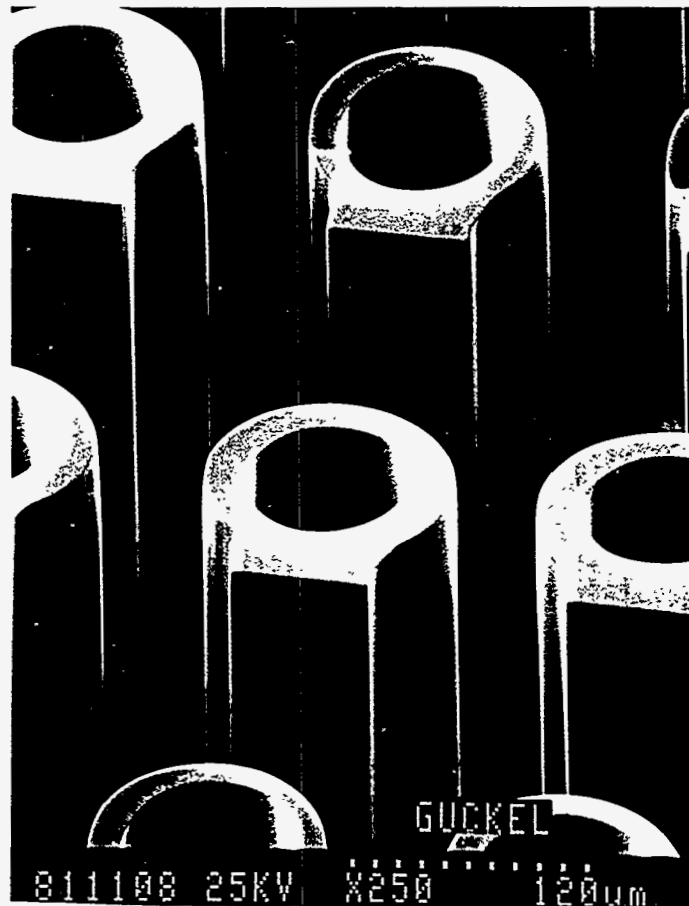
Fig. 2 Developed PMMA test structures 3.2 mm thick exposed with 2.5 GeV synchrotron radiation at the National Synchrotron Light Source of Brookhaven National Laboratory.
