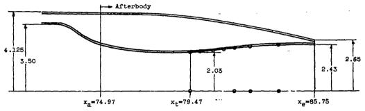
(b) Nozzle 2 (uniform exit). Design pressure ratio, 5.7.
