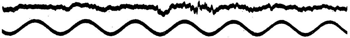
FIG. 3 OSCILLOGRAPHIC RECORD OF TURBULENCE IN THE FREE STREAM.
