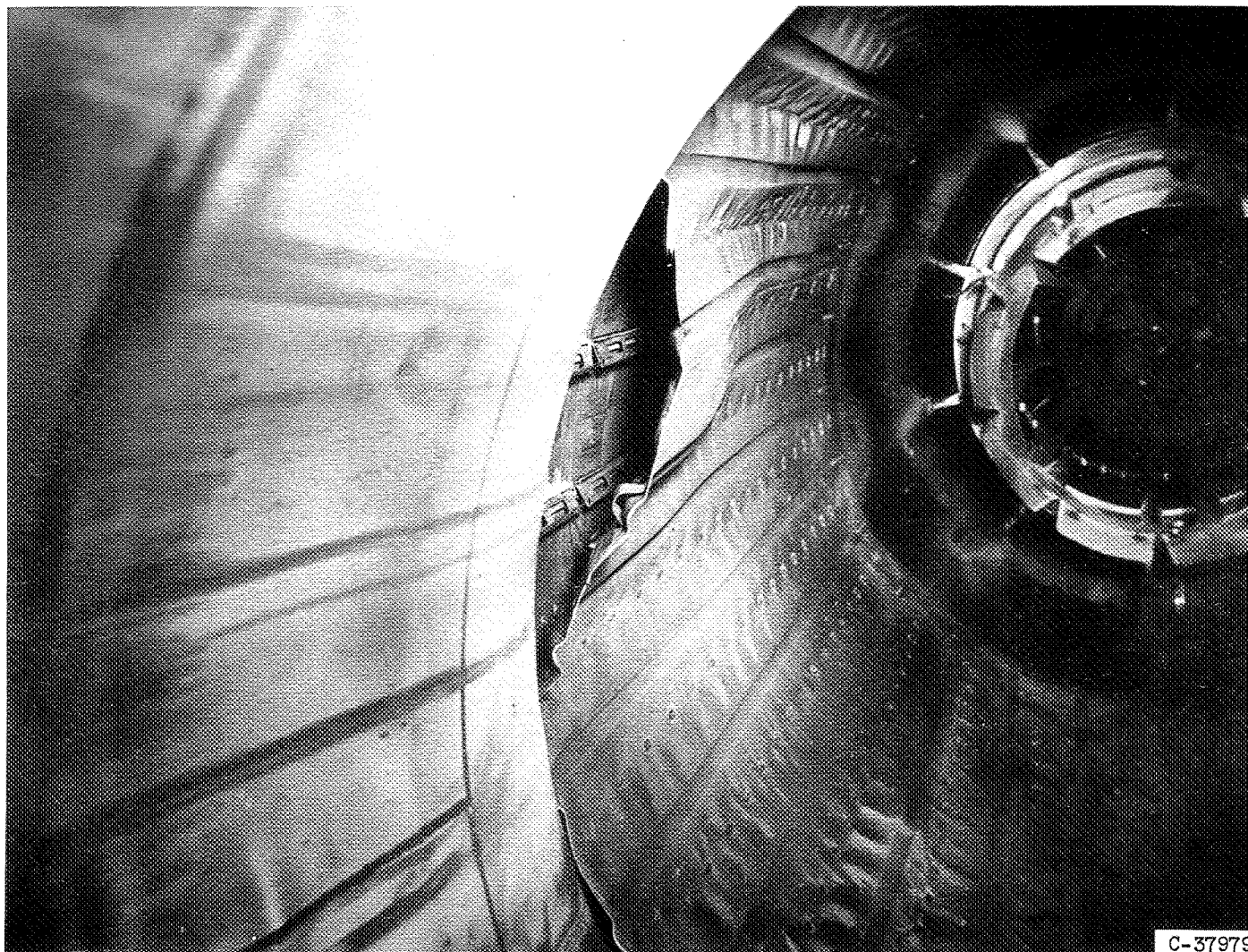
Figure 16. - Failure of third cooling liner after a total burning time of 1 hour and 43 minutes.
