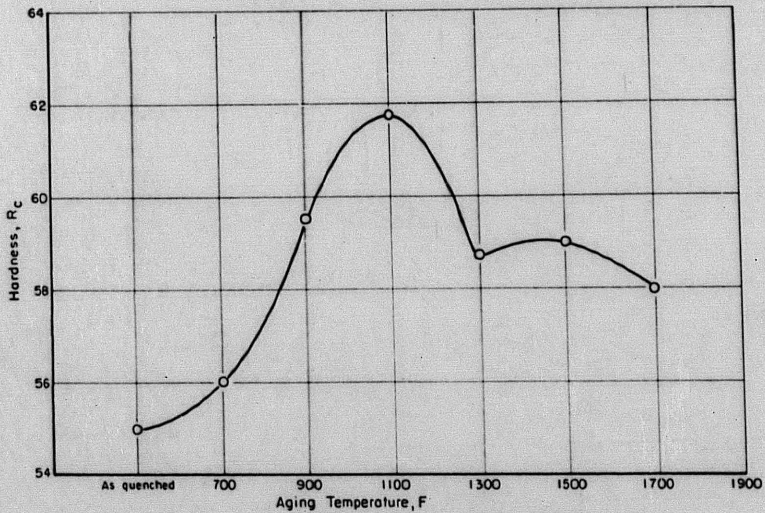
FIGURE 3. AGING EFFECTS IN GE-62 BRAZING ALLOY Specimens solution treated at 1900 F for 5 hr, water quenched, and aged for 5 hr at various temperatures
