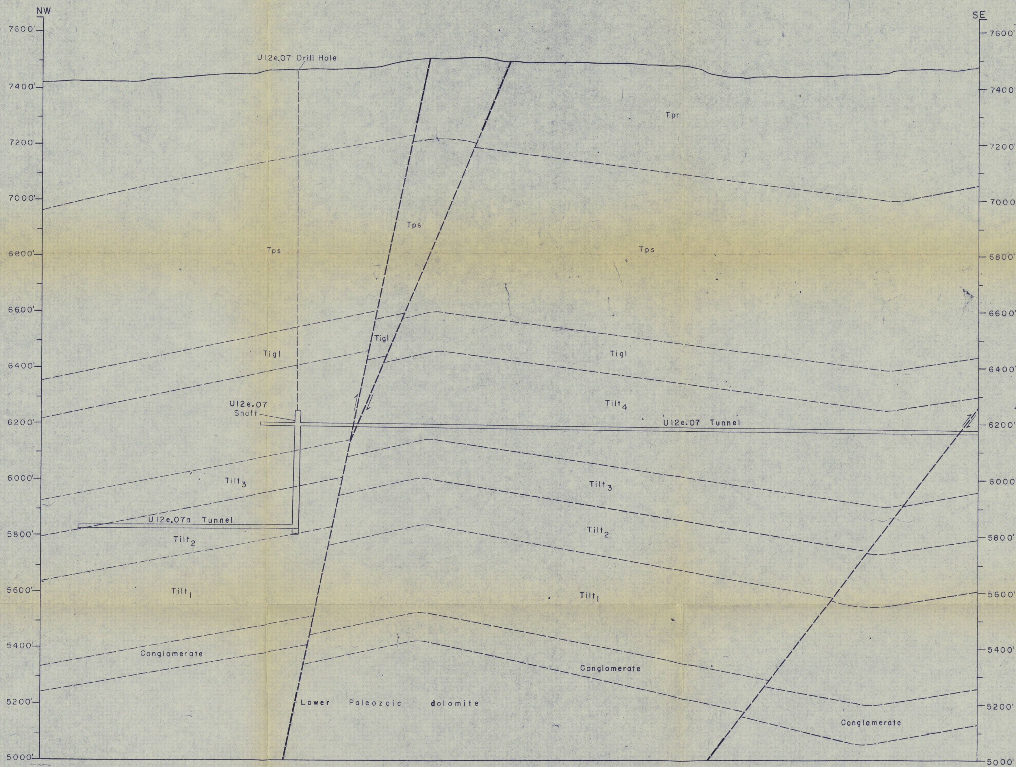
FIGURE 4.-GEOLOGIC CROSS SECTION S.23°03'59"E. THROUGH U12e07 TUNNEL AND SHAFT AND U12e.07a TUNNEL, RAINIER MESA, NEVADA TEST SITE, NYE COUNTY, NEVADA
