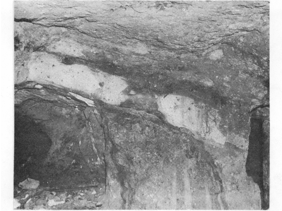
Figure 7. Ore minerals with a double C-roll configuration connecting two mineralized layers. Ore is partly oxidized.
