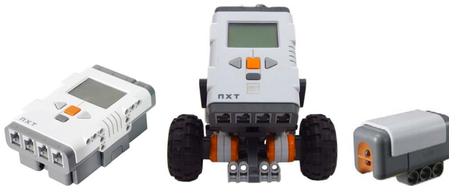
Figure 1: LEGO® MINDSTORMS® NXT: NXT Brick, NXT-Robot, light intensity sensor.
