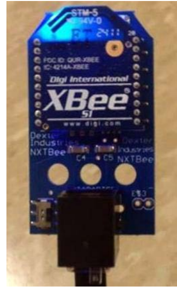
Figure 4: NXTBee communication point to multipoint communication
