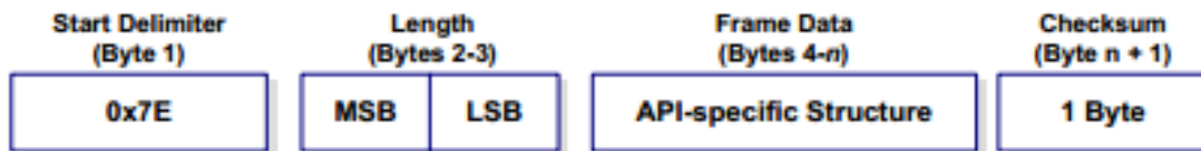
Figure 4.5: ZigBee API Frame Structure
