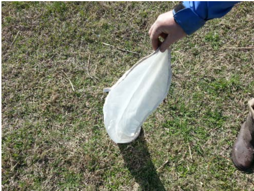
Figure 2.12. Epiphytic macroinvertebrate nylon net (250 \mu\text{m} ) sampling device
