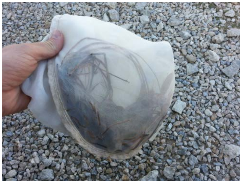
Figure 2.13. Epiphytic macroinvertebrate nylon net (250 \mu\text{m} ) sampling device with American pondweed sample and associated fauna
