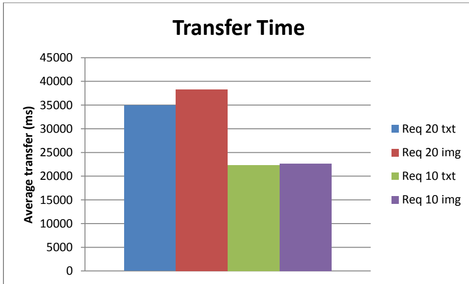
Figure 26. Page transfer time average across all trials for 20 and 10 second timeouts for both text and image pages.
