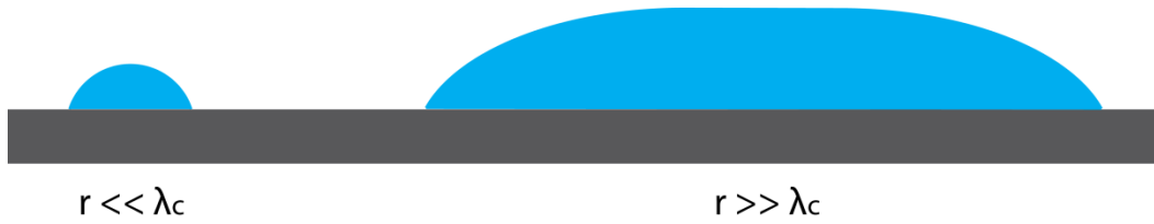
FIG. 2.2 Effect of capillary length on drop morphology
