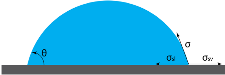
FIG. 2.4 Young's contact angle and surface forces at contact line
