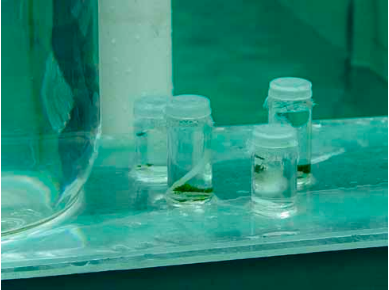
Figure 2. Egg incubation containers with 100 \mu m mesh plastic bolting cloth held over openings with modified lids. Living Stream® in background.
