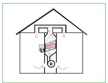
exchanger and heat it up. The gases are then released outside through a vent pipe.
