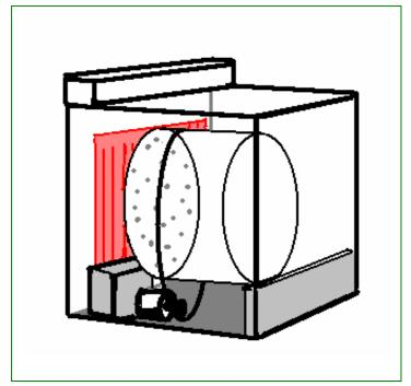
lint screen and through a fan that forces it outside through an exhaust vent.
