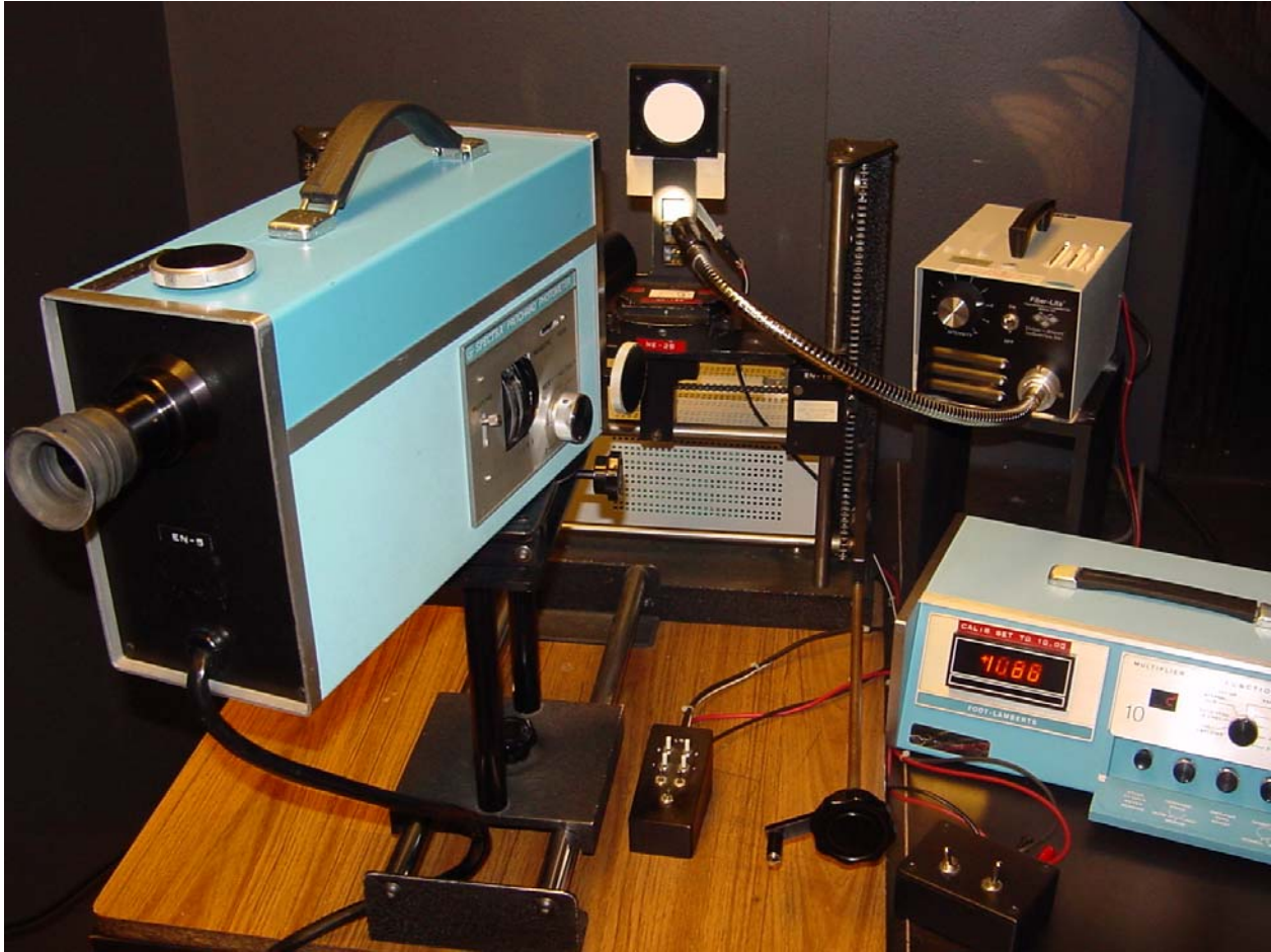
Fig. 9. Test setup for contrast measurements.
