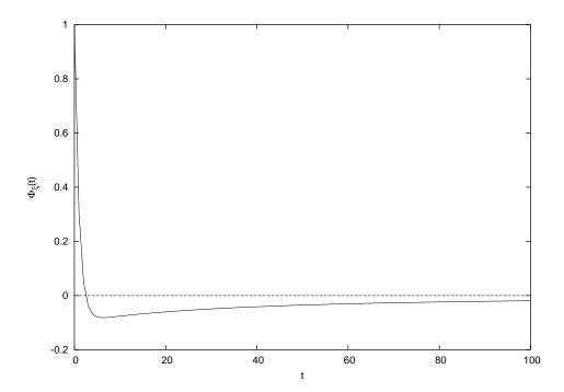
Figure 2.1: The correlation function  $\Phi_{\xi}(t)$  of Eq. (2.67) (full line) and the constant of zero value (dashed line). Here  $\epsilon=0.1,\ \gamma=1,\ T=50$  and  $\beta=1.5$ .
