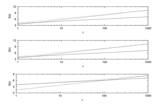
Figure 5.2: The diffusion entropy, S(t), as a function of time t, in a logarithmic scale. Each frame shows three different curves, concerning noise, solid line, slow component, dashed line, and sum of noise and slow component, dotted line. As far as the slow component is concerned, from the top to the bottom frame are shown the results concerning  $SS_J^T$ ,  $SC_J^T$ , and  $SL_J^T$ .
