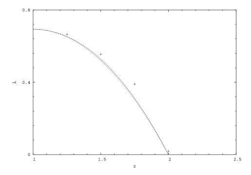
Figure 4.2: The Lyapunov coefficient  $\lambda$  as a function of the parameter z. The dots denotes the results of numerical evaluation, the full line and the dotted line, coinciding in this scale, denote respectively the results of the numerical integration of Eq. (4.25) and the function  $\lambda(z)$  of Eq. (4.26).
