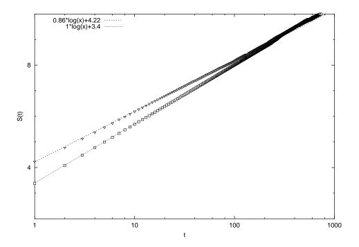
Figure 5.4: The diffusion entropy S(t) as a function of time t, in logarithmic scale. The squares denote the time series corresponding only to the slow component  $SS_j^T$  and the triangles denote the slow component  $SS_j^T$  plus noise. Two straight lines suggest that in the time range from 10 to 100 the former and the latter curves correspond to  $\delta = 0.86$  and  $\delta = 1$ , respectively.
