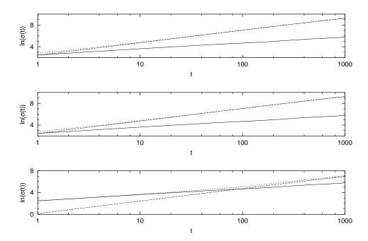
Figure 5.3: The logarithm of the standard deviation,  $\ln(\sigma(t))$ , as a function of time t, in a logarithmic scale. Each frame contains a set of three curves, the full line referring to the noise alone, the dashed line to the slow component alone and the dotted line to the sum of slow component and noise. From the top to the bottom frame these sets of curves refer to  $SS_J^T$ ,  $SC_J^T$  and  $SL_J^T$ , respectively.
