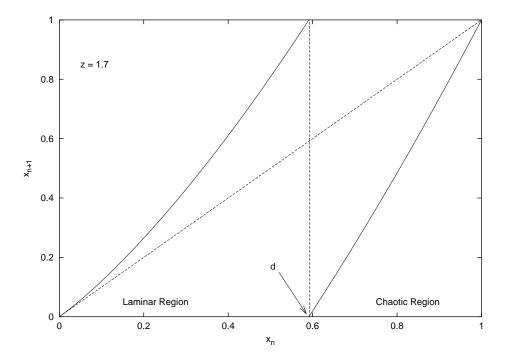
Figure 4.1: The Manneville (full line) map for z=1.7.. The vertical dashed line at  $d\approx 0.59$  divides the phase space in Laminar and Chaotic region. Shown in the picture also the Identity transformation (oblique dashed line).
