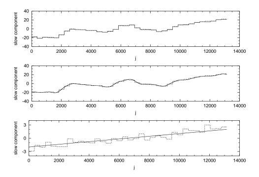
Figure 5.7: The step smoothing technique of Section 5.1.4 at work. The dashed line indicates the results of the step smoothing procedure, and with the full line the slow component to derive. From the top to the bottom frame is represented the case where the slow component are  $SS_j^T,SC_j^T$  and  $ST_j^T$ , respectively .
