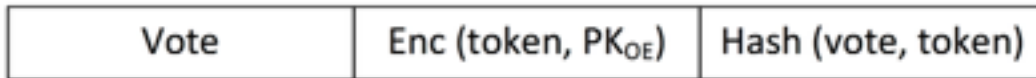
Figure 4.2: A ballot structure. A vote part consist a chosen candidate. Then it followed by a ciphertext, a token encrypted by the public key of election officials. Last field, is a hash of the vote and the token.
