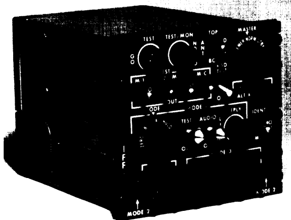
A typical Mark XII airborne transponder. IFF formats and protocols can be handled by any of several types of interrogators and transponders.
