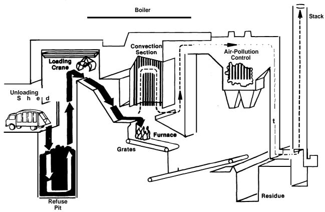
Figure C-1.—Typical Waterwall Furnace for Unprocessed Solid Waste
