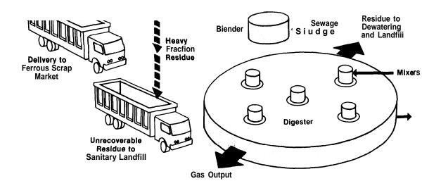
ing tanks, with the remainder discharged to a city sanitary sewer system, The remaining solids, about 17 percent of the refuse feed, must be either landfilled or burned in specially designed boilers. Schulz (6) estimates that approximately 3,700 cubic feet of methane will be produced per ton of MSW.
