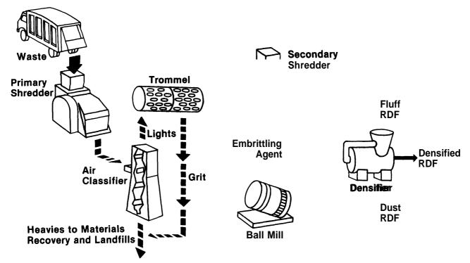
metals and other heavy organic and inorganic materials. The light material then goes through a rotating screen or "trommel" to remove abrasive fine sand, glass, and grit. The heavy materials from the air classifier and trommel move to a magnetic separating device that recovers ferrous material. Some plants also attempt to recover aluminum, glass, and mixed nonferrous metals, using processes described in a later section.
