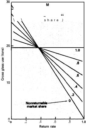
Figure 20.—Glass Required to Deliver a Total of 1 Million Ounces of Soft Drinks in a Mix of Refillable Bottles and Cans if the Nonreturnable Glass Market Share Is Zero and No Glass Is Recycled
