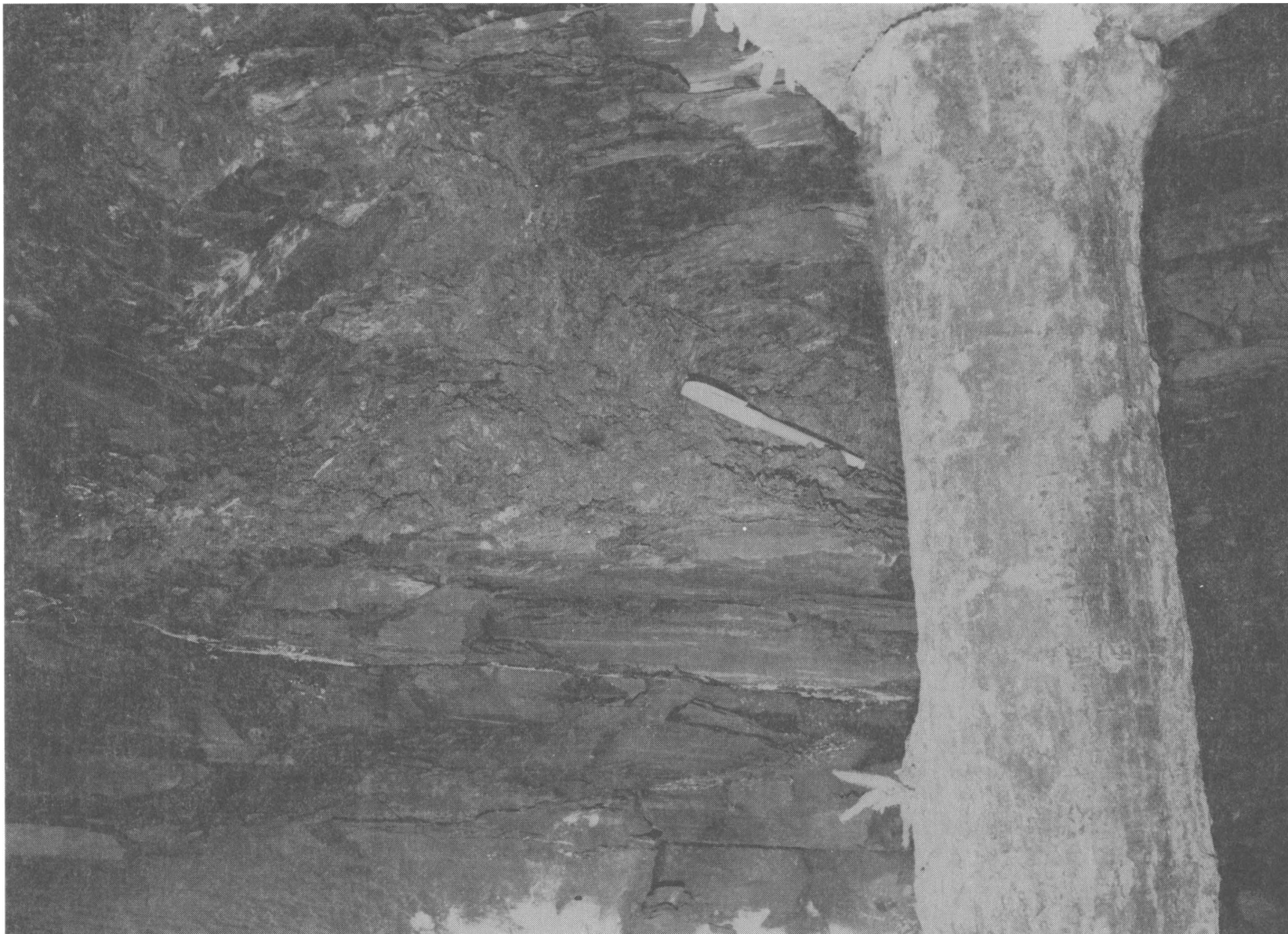
FIGURE 20. - Photograph of thrust fault showing 1- to 3-inch (2.6- to 7.7-cm) fault gouge along thrust plane.
