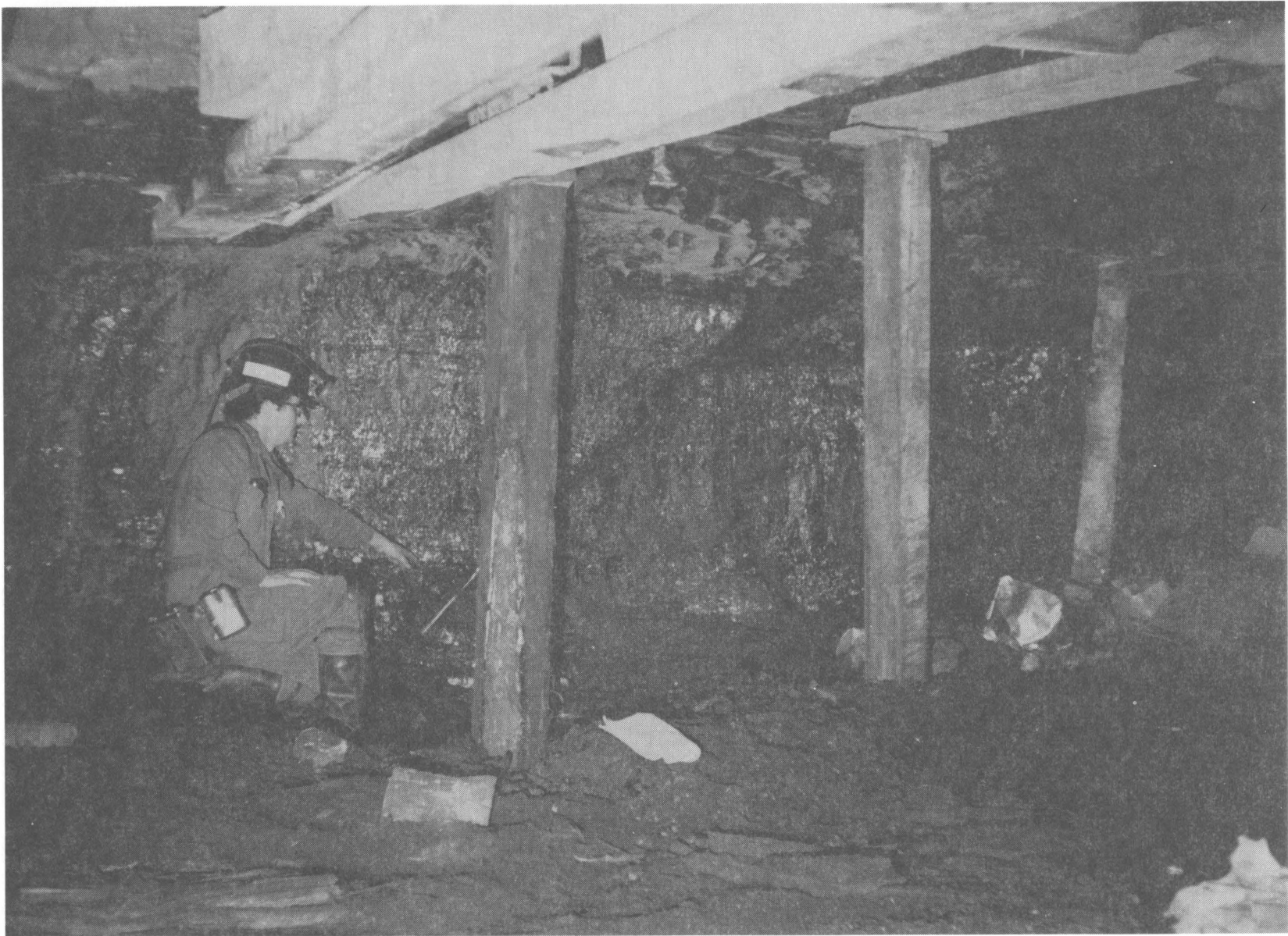
FIGURE 21. - Photograph of thrust fault cutting across the Upper Kittanning Coalbed at a 45° angle.
